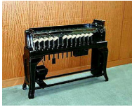
This is the first horizontal card sorter, introduced by IBM in 1925 to operate at about twice the speed of the older Type 70 vertical sorter. This machine uses a direct magnetically operated control for the shoe reader which replaced a much more complex mechanical device in the older machine. The Type 80 grouped all cards of similar classification (such as "sales by product") and at the same time arranged such classifications in numerical sequence. With 10,200 units on control at the close of 1950, the Type 80 had the largest inventory for any machine at that time. http://www-03.ibm.com/ibm/history/exhibits/ibm3/ibm3_136.html
