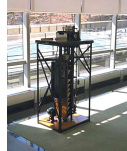
The original Hollerith electric tabulating system did not have an adequate method for sorting cards. This became a problem in the 1930 agricultural census, so Herman Hollerith (1860-1929) developed an automatic sorter. The first one was a hobby model with the bars arranged horizontally. Later, when his system was gaining favor commercially, Hollerith redesigned the sorter into a smaller, vertical machine that would not take up too much space in small central offices. The 070 Vertical-Sorting Machine of 1966 could operate at a rate of 250-370 cards a minute.
