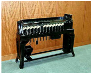
This is the first horizontal card sorter, introduced by IBM in 1925 to operate at almost twice the speed of the older Type 70 vertical sorter. This machine uses a direct magnetically-operated control for the slide flukes which replace a much more complex mechanical device in the older machine. The Type 80 grouped all cards of number classification (such as "tabular products") and at the same time arranged such classification in numerical sequence. With 10,200 units on a card at the close of 1943, the Type 80 had the largest memory for any machine at that time.
